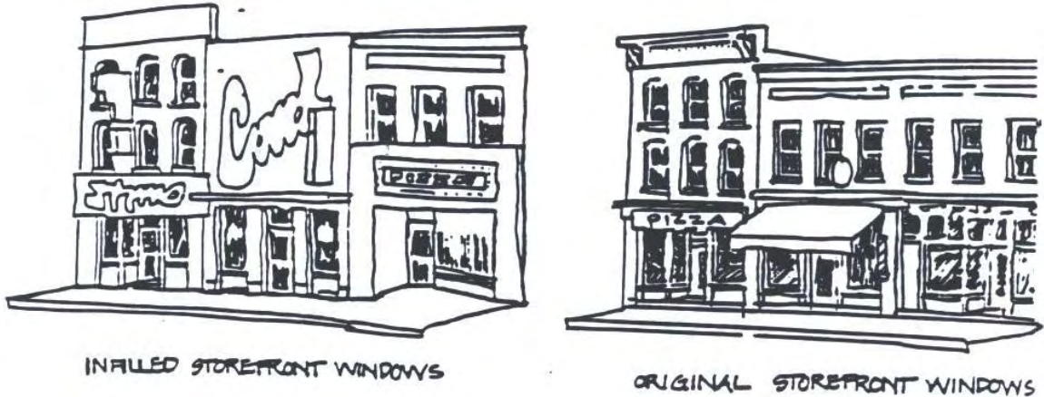
Illustration 20.2 Avoid Attempts at Hiding an Older Façade.
